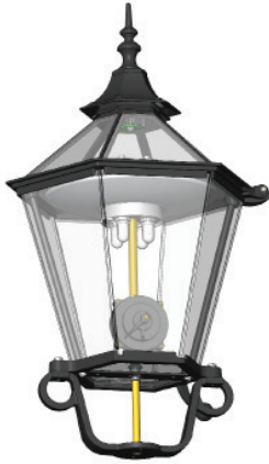
Before the start of the reconstruction, the lamp was completely captured with modern CAD software
